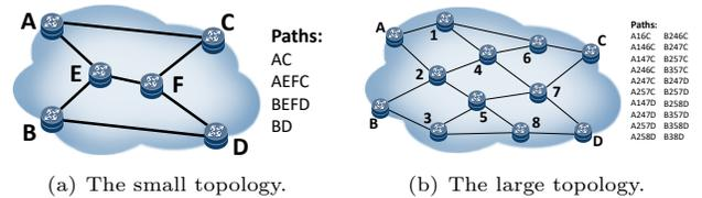
**Figure 4: The packet routing environment. The large topology has the same complexity as the real Abilene Network<sup>4</sup> in terms of the numbers of routers, links and paths. It is used for scalability test.**
